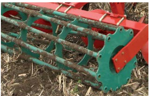
Kavezasti valjak ø 550mm, 90kg/m
