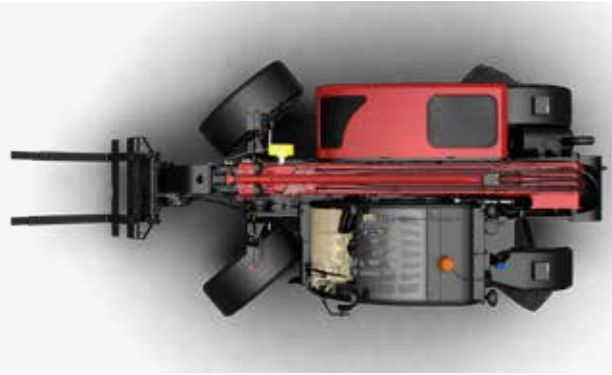
Four wheel steer: minimises the Farmlift's turning cycle and maximises manoeuvrability.
